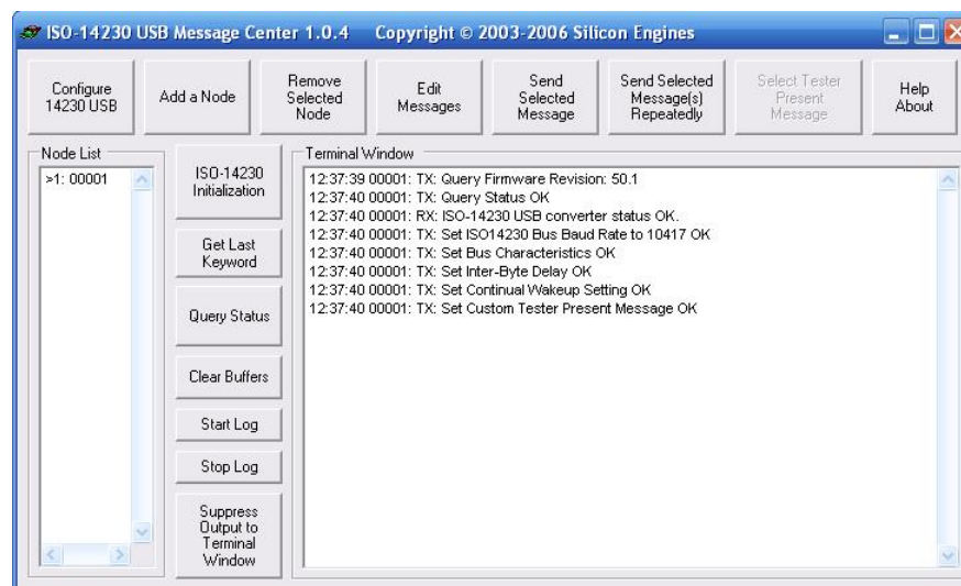
QUERY STATUS BUTTON SHOWS FIRMWARE REVISION FIGURE 21.2.1
